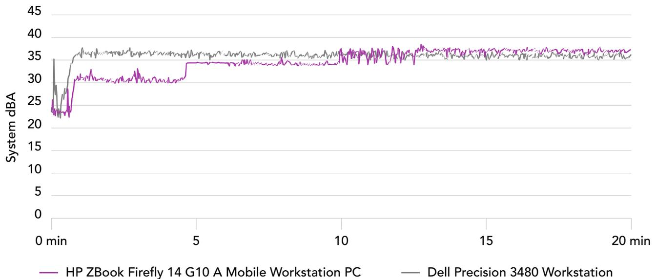
Figure 1: Acoustic testing results, in A-weighted decibels. Lower is better. Source: Principled Technologies.
