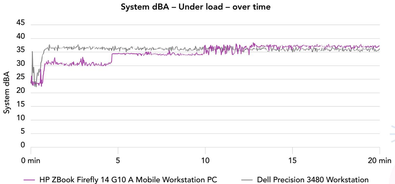
Figure 8: Acoustic testing results, in A-weighted decibels. Lower is better. Source: Principled Technologies.
