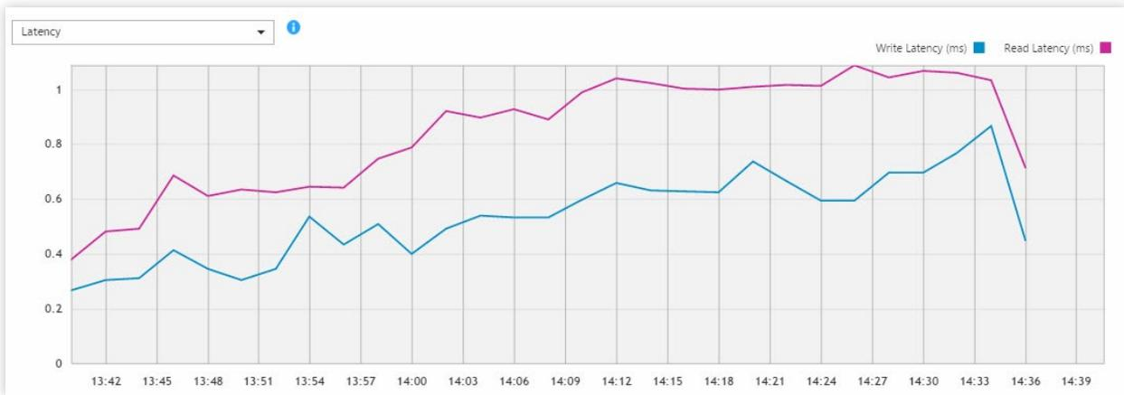
With the additional fourth node, the upgraded environment latency peaked at just over a 1.6ms read and a 1.1ms write. Again, latency remained at around 1 ms.
