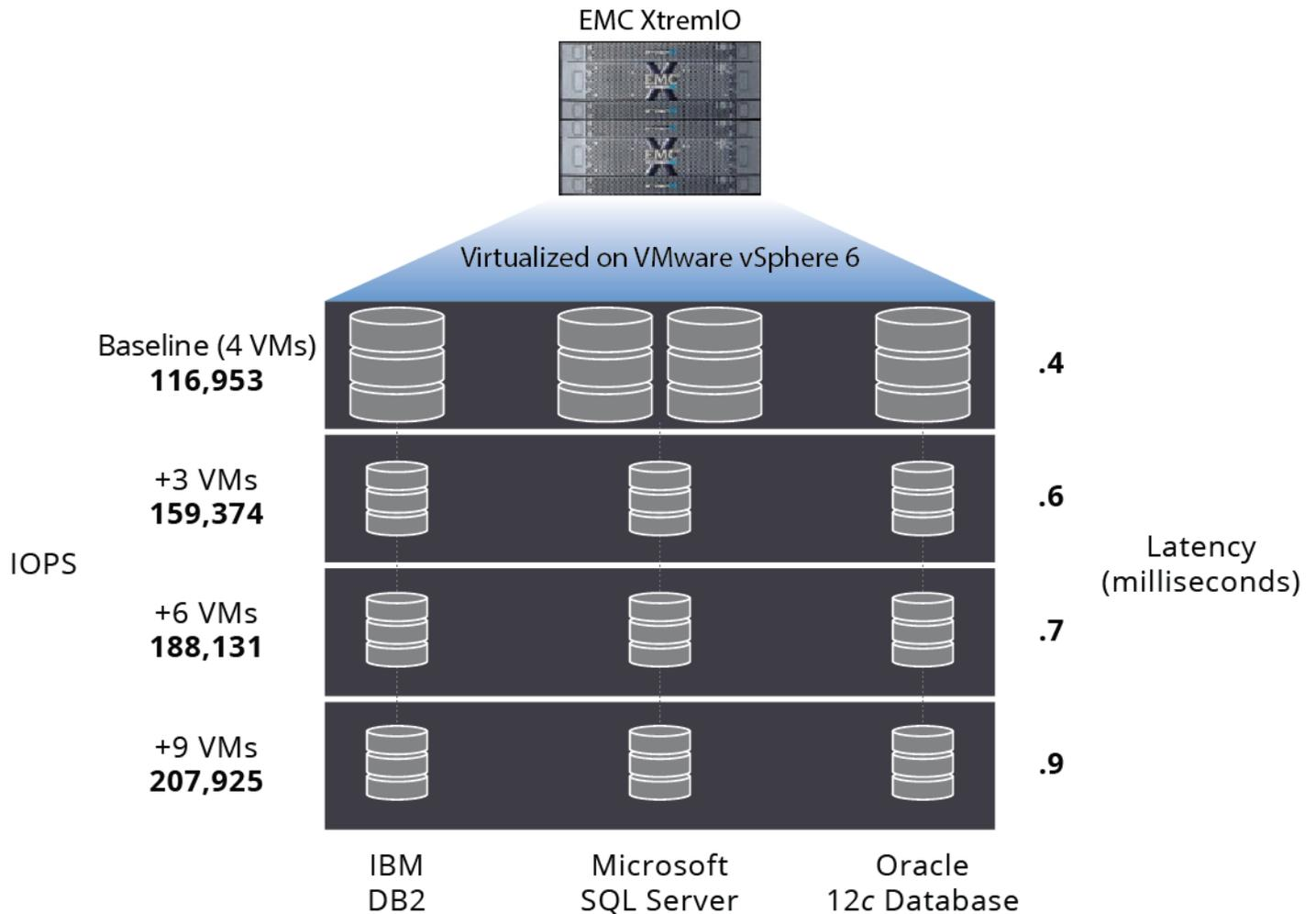
Figure 2: Testbed configuration overview with IOPS and latency results.
