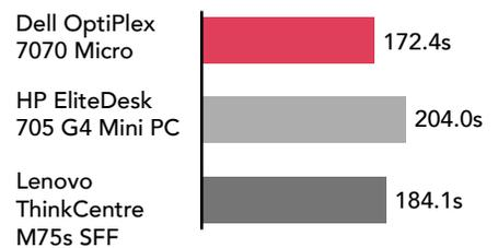
Figure 9: Rendering a 4K RED video file to H.264. Time (sec). Lower is better. Source: Principled Technologies
