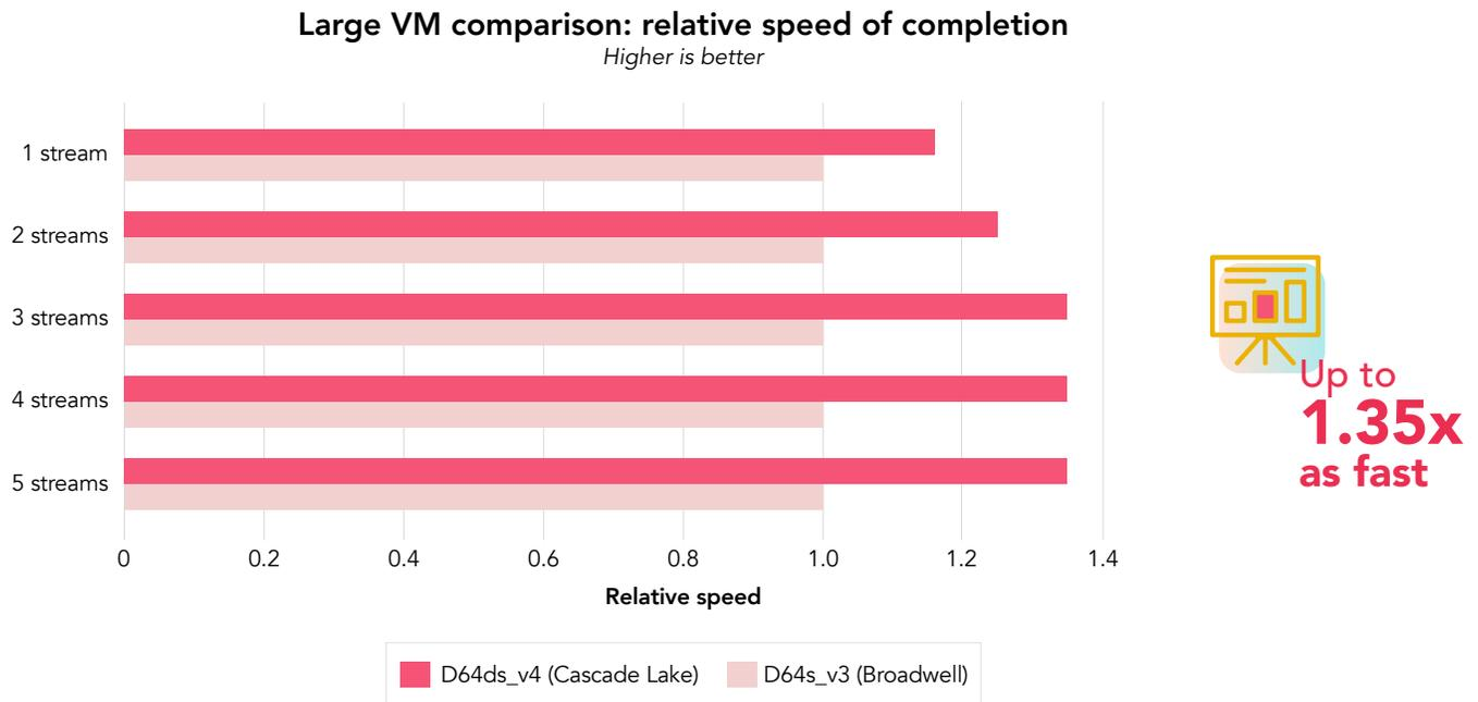
Figure 3: Comparison of the relative speed at which each large VM completed one, two, three, four, and five query streams from the TPC-H-like HammerDB workload. Greater speed is better. Source: Principled Technologies.
