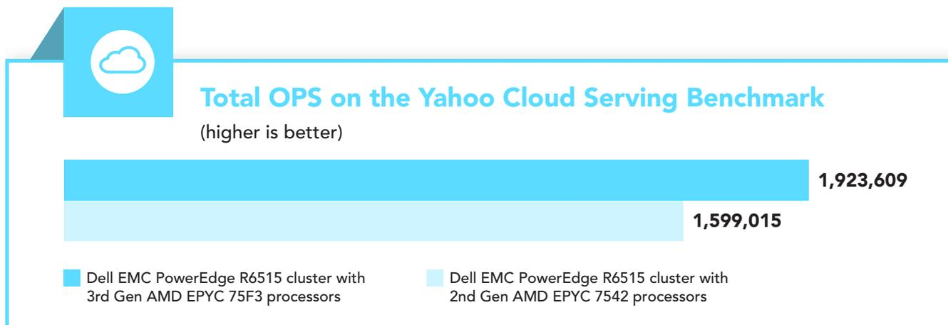
Figure 2: Total number of operations per second each cluster achieved in testing on YCSB Workload C. Higher is better. Source: Principled Technologies.
