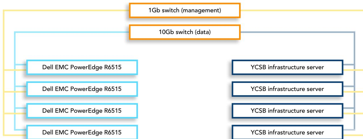
Figure 1: The testbed we used. Source: Principled Technologies.
