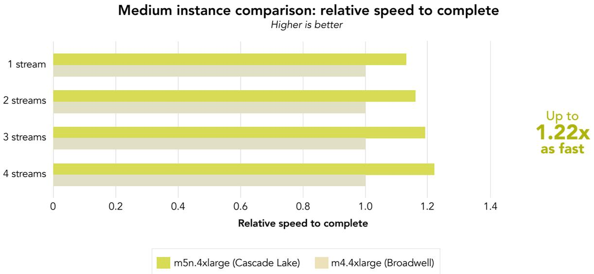
Figure 2: Normalized comparison of the speed at which each medium instance completed one, two, three, and four query streams from the TPC-H-like HammerDB workload. Higher speed is better. Source: Principled Technologies.
