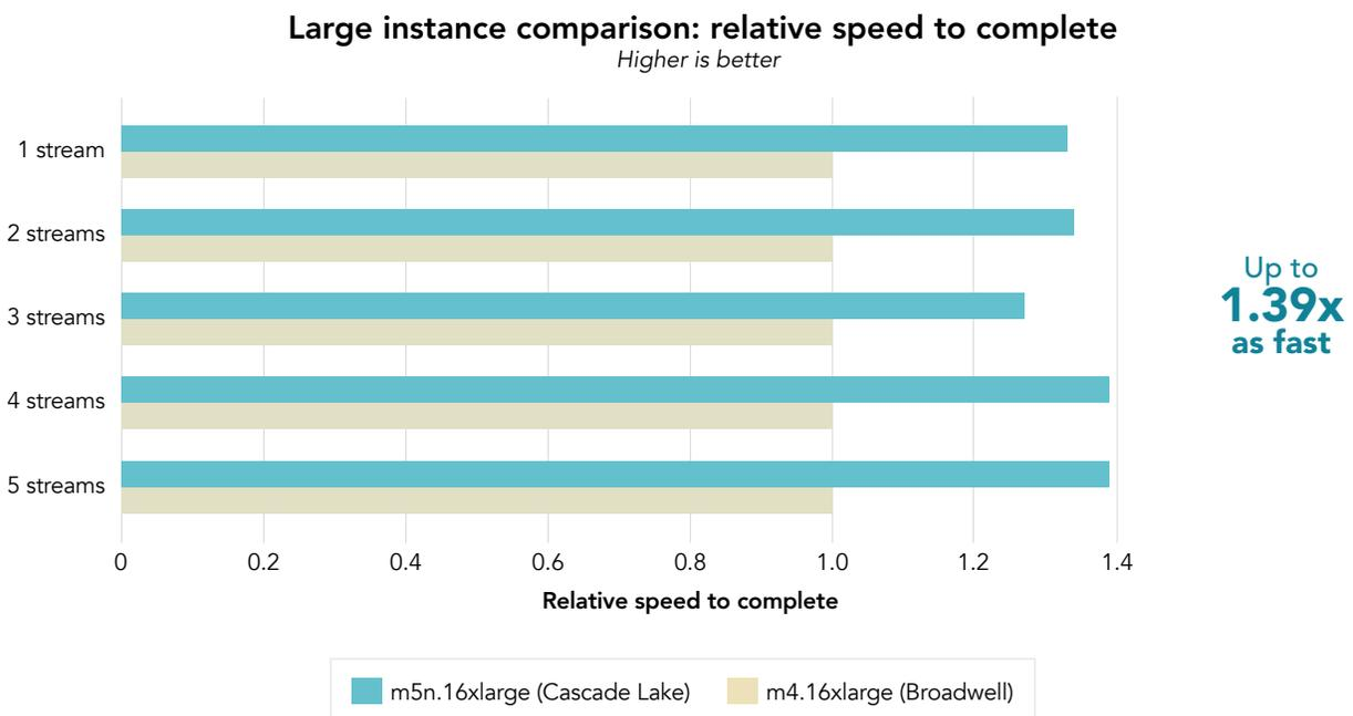
Figure 3: Normalized comparison of the speed at which each large instance completed one, two, three, four, and five query streams from the TPC-H-like HammerDB workload. Higher speed is better. Source: Principled Technologies.
