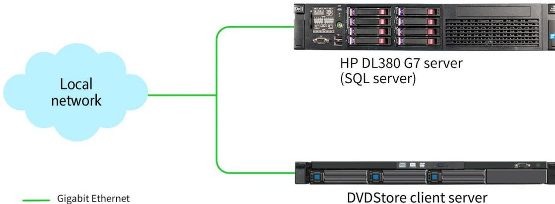
Figure 7: The testbed diagram for the legacy solution.
