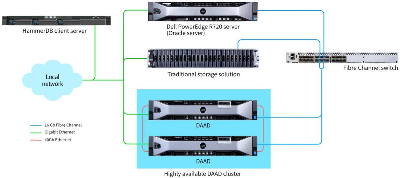
Figure 4: The combined traditional storage/highly available DAAD configuration we tested.
