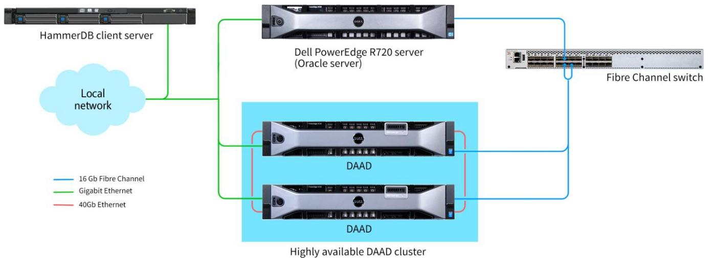
Figure 5: The highly available DAAD configuration we tested.
