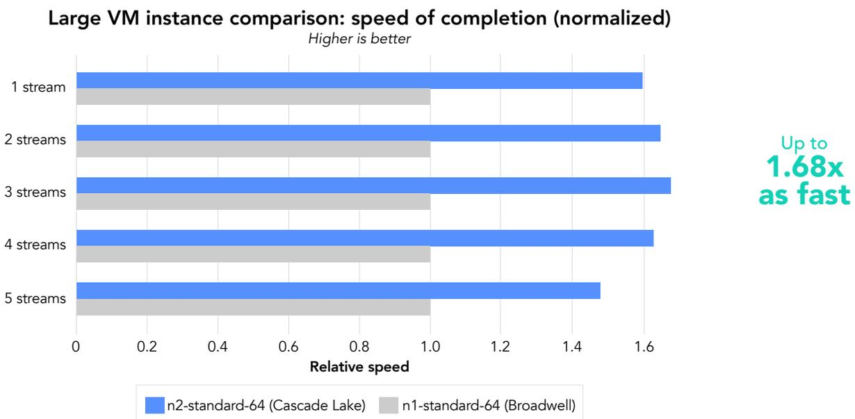
Figure 3: Comparison of the speed at which each of the large VM instances completed the TPC-H-like workload from HammerDB, relative to the completion time of the n1-standard-64 VM instance. Greater speed is better. Source: Principled Technologies.
