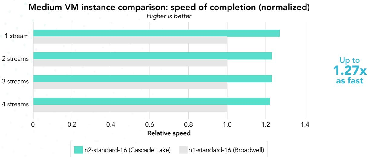
Figure 2: Comparison of the relative speed at which each of the medium VM instances completed the TPC-H-like workload from HammerDB, relative to the completion time of the n1-standard-16 VM instance. Greater speed is better. Source: Principled Technologies.
